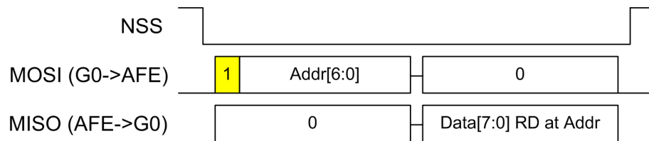
Figure 68. Single byte read access
