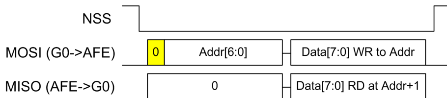
Figure 67. Single byte write access
