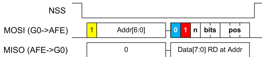
Figure 74. Read Modify Write access
