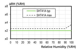
**Figure 2.** SHT40A typical and aximal relative humidity accuracy at 25 °C.
