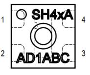
**Figure 12.** Pin assignment (transparent top view). Dashed lines are only visible if the sensor is viewed from below. The die pad is not directly connected to any pin.
