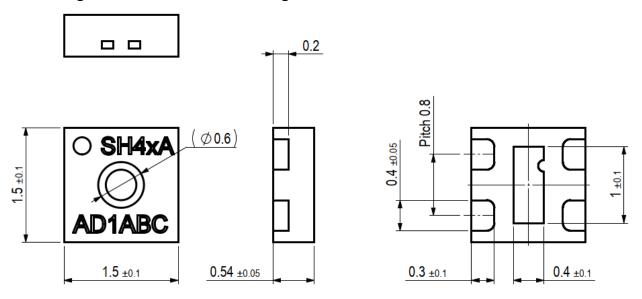
Figure 10. Dimensional drawing of SHT4xA including package tolerances (units mm).
