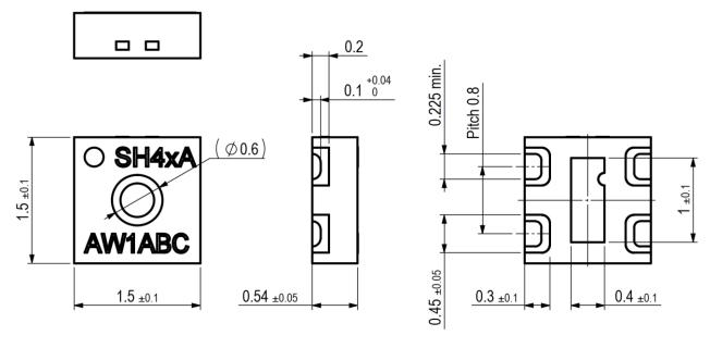
Figure 11. Dimensional drawing of SHT4xA with wettable flanks, including package tolerances (units mm).
