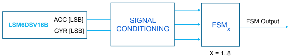
Figure 3. State machine in the LSM6DSV16B
