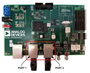
Figure 6. Network Interface Port Location
