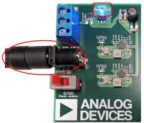
Figure 2. Power Cable Connection and Power Valid LED
