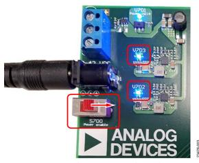
Figure 3. Power Switch in ON position and 5 V and 3.3 V LEDs
