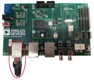
Figure 5. Ethernet Cable Connection
