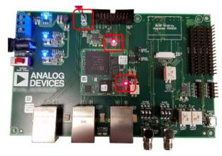
Figure 4. Reset Switch Location and Reset LEDs
